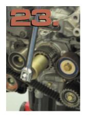
Remove both cam sprocket holding tools, then install the crankshaft turning socket. Turn the crankshaft 90 degrees counterclockwise, then 180 degrees clockwise, before returning the crankshaft sprocket to its alignment mark. This combination of movements allows the tensioner to take the slack out of the new belt and normalizes its position on the assortment of sprockets and idlers.
