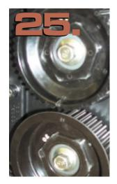
The timing marks on this engine lined up everywhere but here at the left cam sprocket match marks. After normalizing the belt by rotating it, the upper and lower pulley match marks didn't line up quite as precisely as we would have liked. The four marks didn't line up like four fingers pointing directly at each other. Rather, they lined up like four fingers pointing ever so slightly away from each other.
