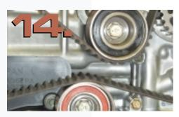
The 2.5 engine's timing belt must negotiate a combination of three idler pulleys, the water pump pulley and the tensioner pulley during each rotation. Pay particular attention to the position and appearance of the different idler pulleys, especially if you happen to
