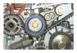
ball and silicone oil. Remove the mounting bolt, then remove the tensioner assembly.
