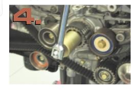
crankshaft, and provides a convenient way to turn the engine over with a breaker bar. Use the tool to turn the crankshaft until all of the timing marks are aligned. This step is especially important because we don't want to try to retime the engine after the timing belt has been removed.
