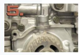
There are seven different timing marks that need to be in alignment. Close doesn't count here — we're not playing horseshoes. We'll start with the crankshaft pulley. Make sure the timing mark on the crankshaft reluctor is lined up with the corresponding mark on the engine case.
